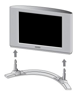
Note: The curved side of the stand base should be placed at the back of the TV set as shown in the above figure.
